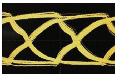
Bad eye-pattern of AES/EBU signal after 100 ft of standard microphone cable
